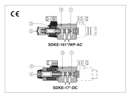
Spool type, two or three position direct operated valves with threaded solenoids. Solenoids ② are made by:
